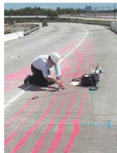
*Testing for quality of grout injection in cable ducts located by ground penetrating radar*
