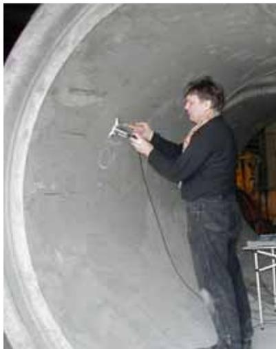
*Detection of delaminations and honeycomb in sewer pipe*
