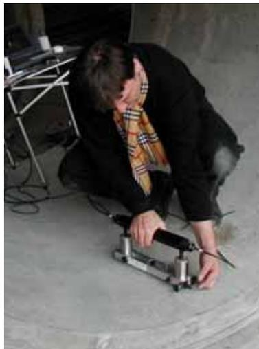
*Measurement of P-wave speed by surface method*
