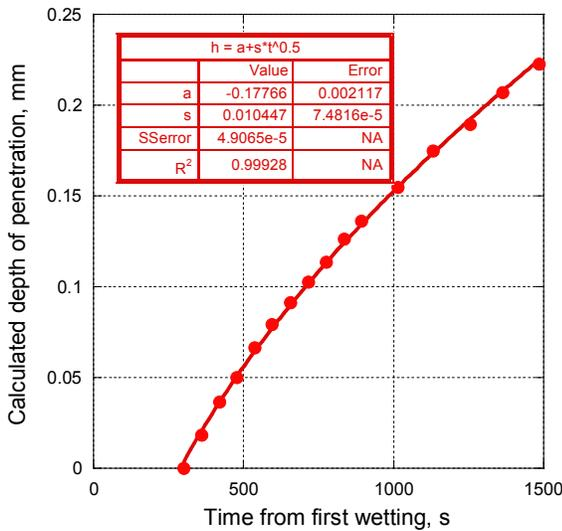
It has been found that the depth of water penetration is a linear function of the square root of time (1), where time is measured from when water is first added to the GWT chamber. Therefore, the following function can be fitted to the data:
