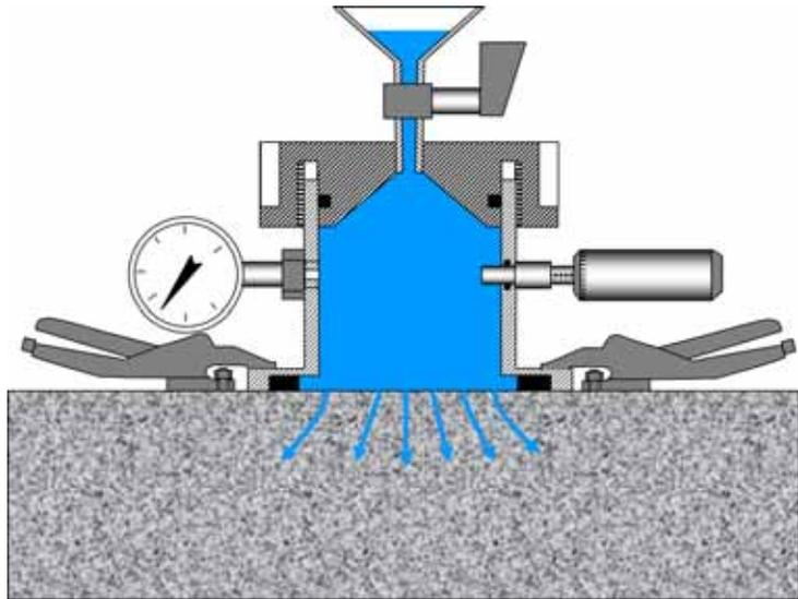
The travel of the piston as a function time is recorded and the speed the piston travel in  $\mu\text{m/s}$  is used to characterize the permeation of the test surface.
