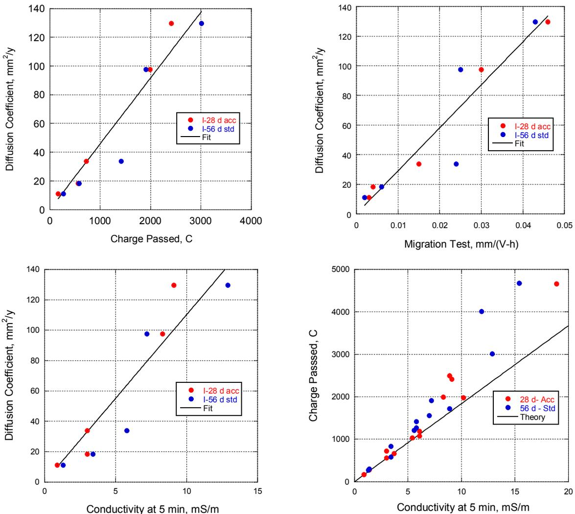
The above plots show that there are strong relationships between the various electrically based test methods and the apparent chloride diffusion coefficient.
