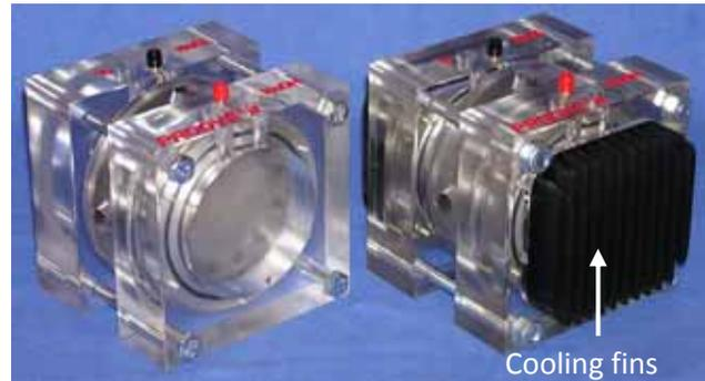
*Two types of PROOVE'it cells: standard PR-1000 cell (left) and PR-1100 cell with cooling fins (right)*
