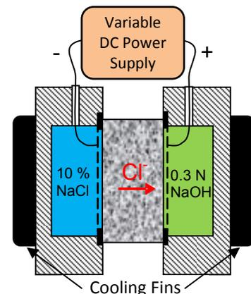
measured by spraying the split surface with a 0.1 M silver nitrate solution, which precipitates as white AgCl where chlorides are present. From the penetration depth and test conditions, the chloride ion migration coefficient is calculated. It is important to maintain a constant temperature in the solutions in the reservoirs. Therefore, cells with cooling fins (Part No. PR-1100) are recommended.
