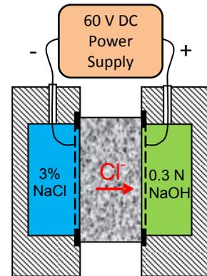
The more permeable is the concrete, the more negative ions will migrate through the specimen, and a higher current will be measured. The current is measured for 6 hours. The area under the curve of current versus time is determined, which represents the total charge or Coulombs passed across the specimen. Test results are corrected for a standard specimen diameter of 95 mm. The Coulomb values are used for classifying the concrete as follows (ASTM C1202):
