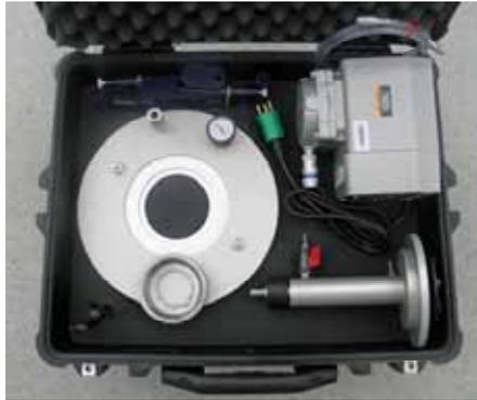
**B-10000 DSV-Kit:** For surface planing, bonding the disc, and attaching the coring rig to produce the partial core without anchoring.
