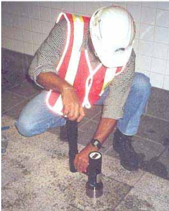
**BOND-TEST** being performed on granite tiles in a subway station
