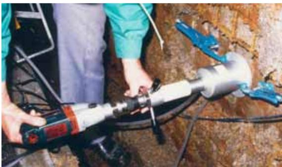
Coring with the **CS-75** rig for inspection of cracks following chloride extraction
