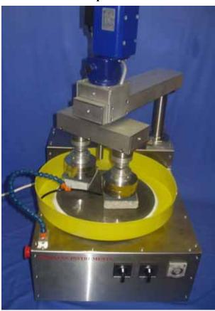
The photo on the left shows the complete **PetroPlaner** unit. Shown below are details of the attachment to the two specimens and the built-in self-feeding and recycling system for the grinding slurry.
